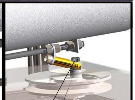
*SHOULDER BOLT*/threads into *PULLEY*, ensure the *SPACER* is in place. Then lightly tighten the rod nuts
