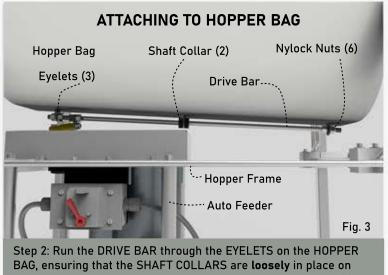
BAG, ensuring that the SHAFT COLLARS are **loosely** in place on **either** side of the center EYELET **before** threading on the NYLOCK NUTS. Adjust the NYLOCK nuts so that the outer EYELETS **spread apart**, then tighten the SHAFT COLLARS around the center EYELET.
